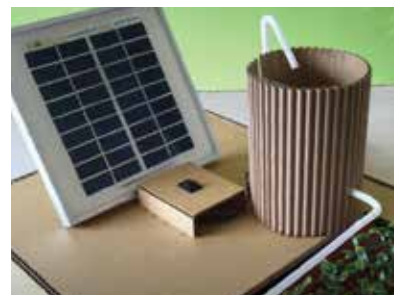
Solar powered plant watering
